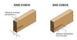
Checking often occurs along the first glue line adjacent to the outer lamination that may dry more rapidly because a larger surface area of that lamination is exposed to the air. This condition is sometimes aggravated when the outer lamination tends to cup, creating tension perpendicular to grain stresses along or near the first glue line.
