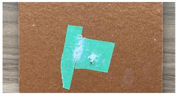
4. Use the brush cap bottle of the base coat (shaking beforehand) and use a small amount of paint product to cover only the filled scratch/gauge.
